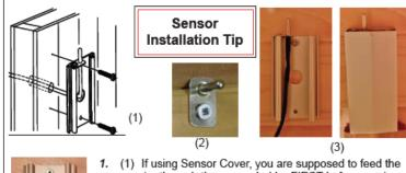
(1) If using sensor cover, you are supposed to read the sensor wire through the sensor holder FIRST before running wire inside the wall. If not done first, do one of the following:
